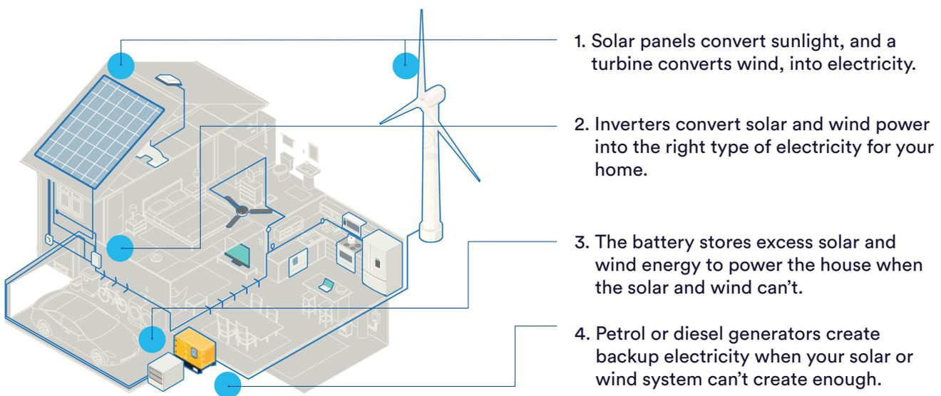
1. Solar panels convert sunlight, and a turbine converts wind, into electricity.
